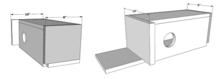
Cut out a 3" door in one of the 16  $\frac{1}{2}$ " pieces, approx. 2  $\frac{3}{4}$ " from the top. This piece may go on on either the right or left side of the 25" back. The roof should overhang the door. The remaining 8" piece is the floor.
